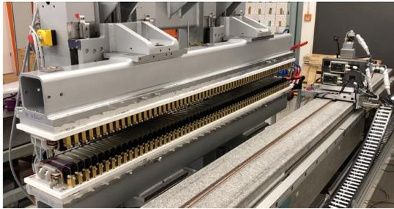
Figure 4: Completed FIR U-68 undulator during magnetic mapping at FHI.
