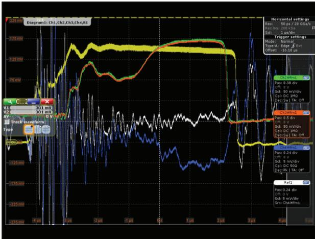
Figure 5: Observation of spontaneous emission with a mercury cadmium telluride (MCT) detector – blue trace.
