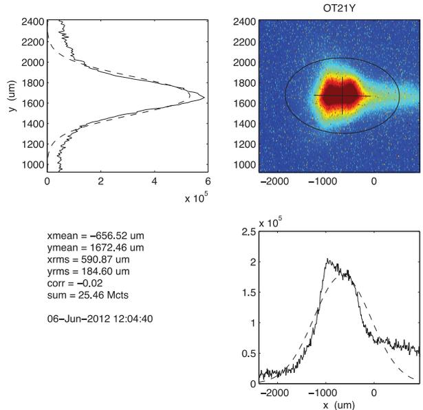
Figure 8: Beam size measurement for the image in Figure 7 representing ~ 0.1% energy spread at 45 MeV.
