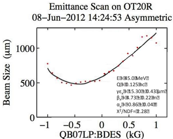
Figure 9: Emittance scan for 125 mA, 45 MeV beam.
