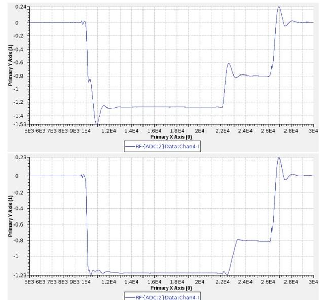
Figure 10: Subharmonic buncher Q signal without (upper) and with (lower) LLRF feed forward.
