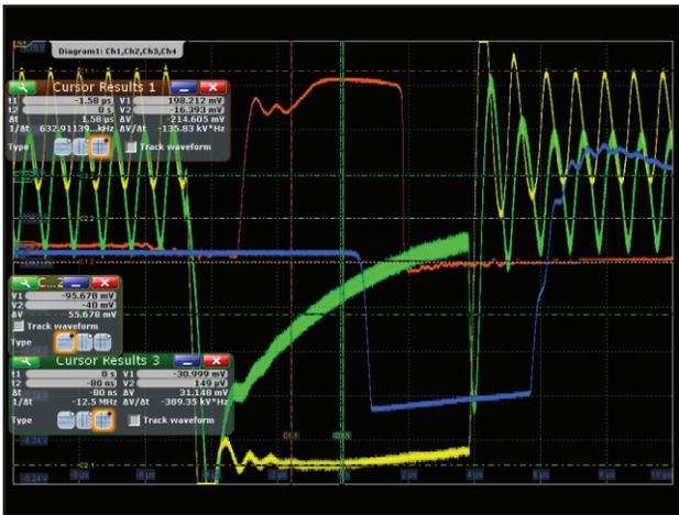
Figure 6: Saturated MCT detector signal in blue confirming first light.
