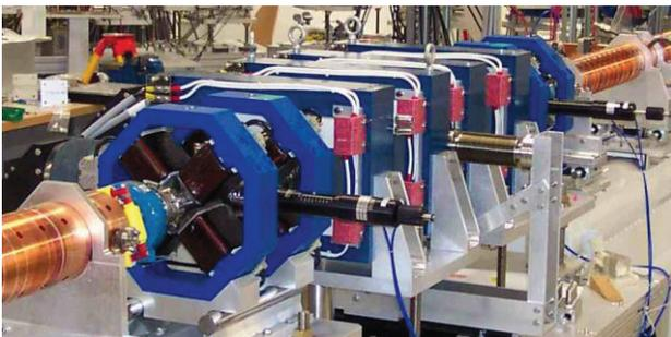
Figure 4: FEL chicane between quadrupole doublets.
