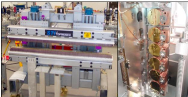
Figure 4: (left) STI Optronics MIR undulator, (right) Bestec mirror changer equipped with 6 gold-coated copper mirrors with different out-coupling hole diameters.
