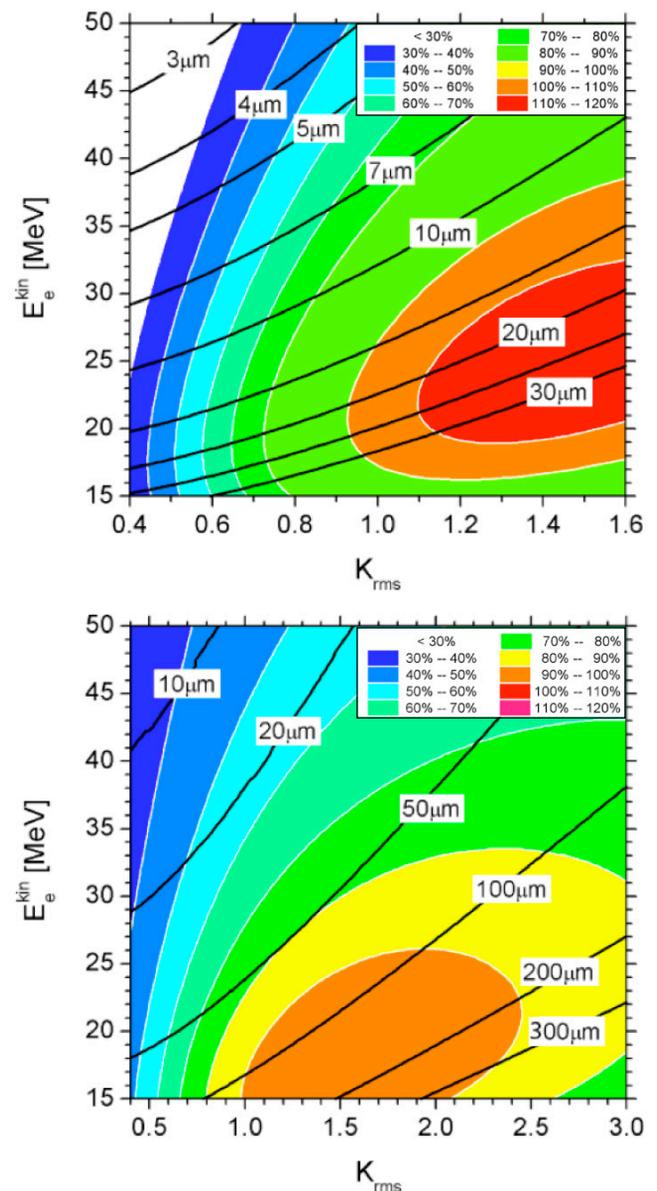
Figure 2: Calculated wavelength and small-signal gain for 3 psec long electron bunches of 50 keV energy spread for (top) the MIR and (bottom) the FIR undulators.
