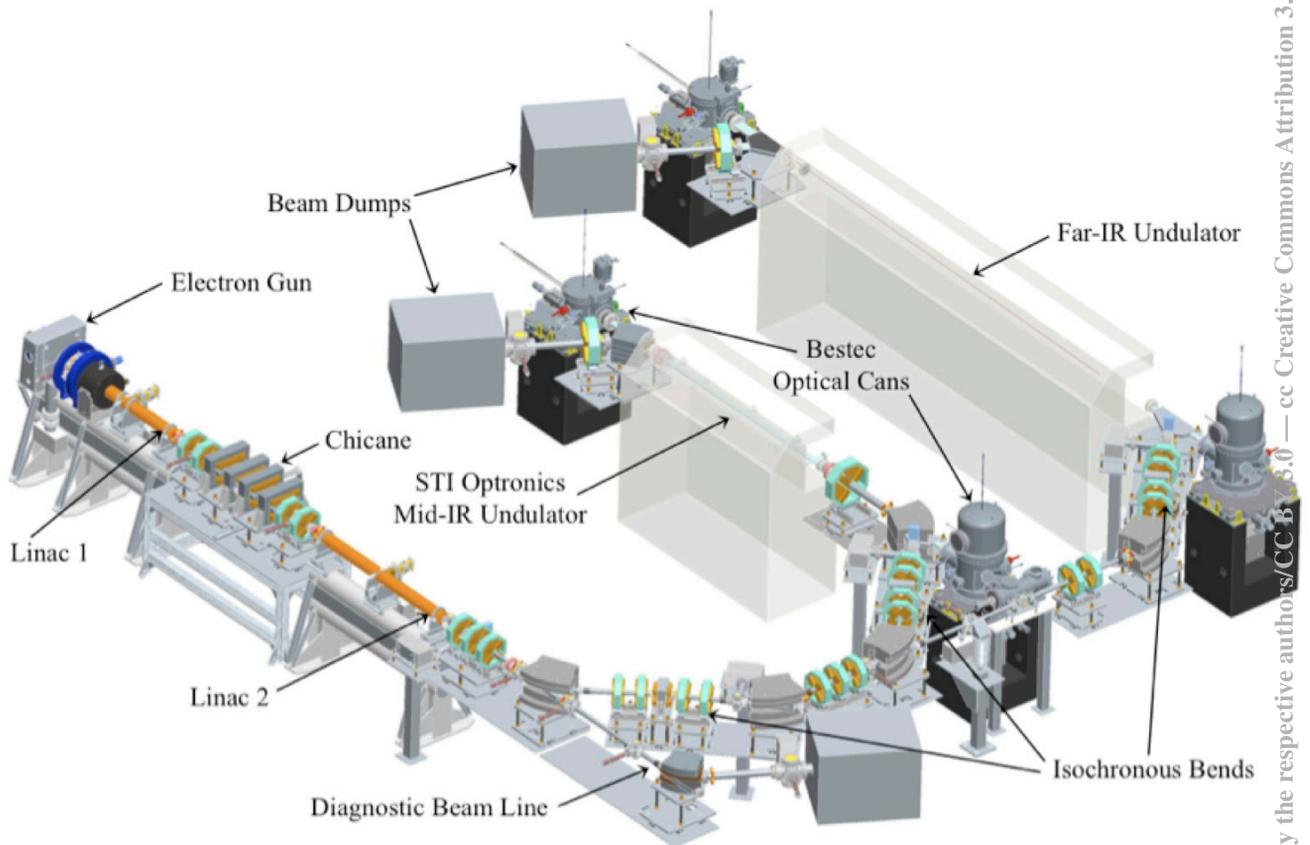
Figure 1: Schematic diagram of Fritz Haber Institute free electron laser showing key components.
