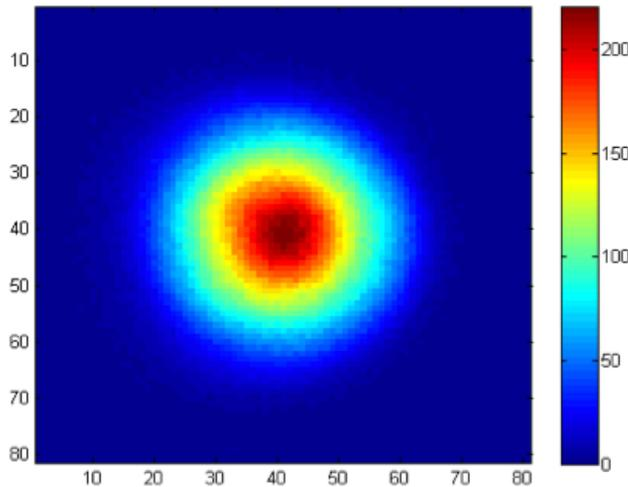
Figure 5: Image of the electron beam spot after pinhole.
