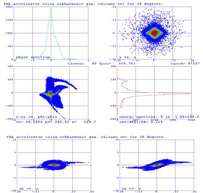
Figure 2: End of Linac 2 electron beam phase space.
