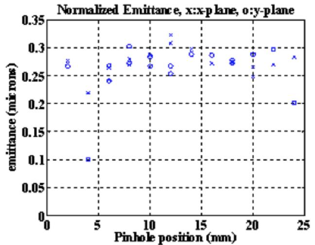
Figure 6: Normalized emittance across the electron beam.
