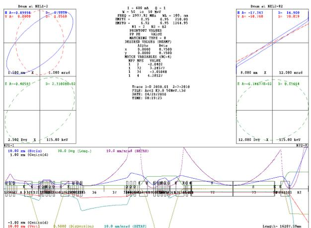
Figure 4: TRACE 3D beam transport line envelopes for the far-IR wiggler with K = 3.0 at 50 MeV.
