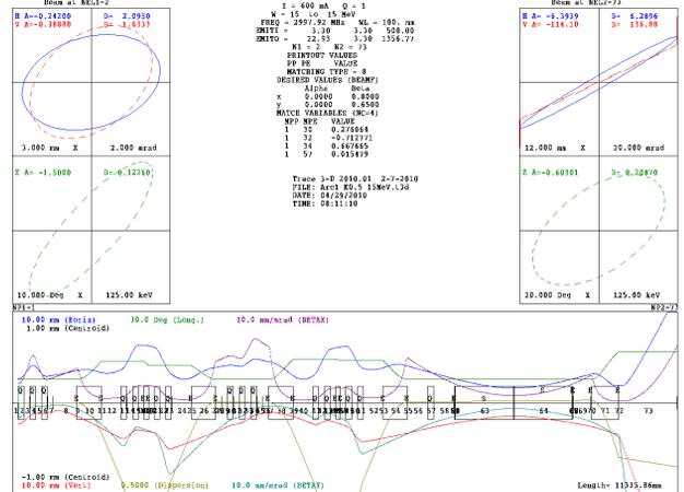
Figure 3: TRACE 3D [4] beam transport line envelopes for the Mid-IR wiggler with K = 0.5 at 15 MeV.
