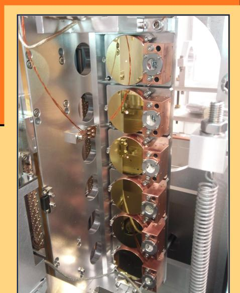
MIR-cavity: wavelength: 4 - 40 μm,
