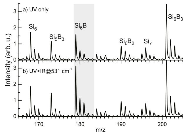
**Fig. 3.** Mass spectra of  $\text{Si}_n\text{B}_m$  clusters irradiated with (a) UV laser only and (b) UV and IR radiation at a frequency of  $531 \text{ cm}^{-1}$ , showing a significant enhancement ( $\sim 70\%$ ) of the  $\text{Si}_6\text{B}$  ion yield with the additional IR radiation.
