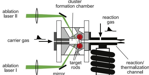
**Fig. 1.** Schematic view of the dual-target dual-laser ablation source for the production of mixed  $\text{Si}_n\text{B}_m$  clusters.
