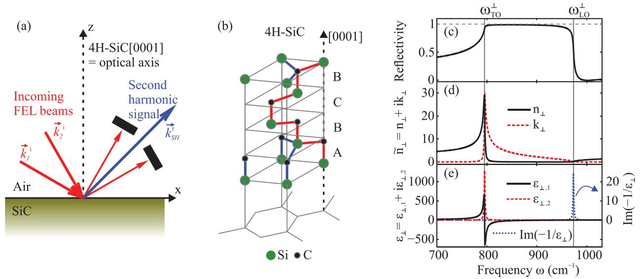
FIG. 1. (a) Schematic of the SHG spectroscopy experiment. (b) Schematic crystal structure of 4H-SiC, also indicating the stacking sequence. (c) Reflectivity in the Reststrahl band, calculated for (d) the complex refractive index and (e) dielectric function of ordinary rays in 4H-SiC.<sup>20</sup> Also shown in (e) is the quantity  $\text{Im}(-1/\epsilon_{\perp})$  that peaks at the zero-crossing of  $\epsilon_{\perp,1}$  (blue-dotted line).
